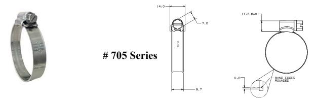
Premium Marine Grade, all AISI 316 (high tensile strength) Stainless Steel Compact "HD NON-PERF" Worm Gear Hose Clamp. The 9.7 mm (0.382") wide band is Non-Perforated and Smooth on the inside with Rolled Edges. This eliminates hose damage with increased clamping force. The High Strength, Compact, One Piece 14mm (0.55") wide Housing provides one of the highest clamping force ratings of any worm gear style clamp. Screw Head is 7mm.
